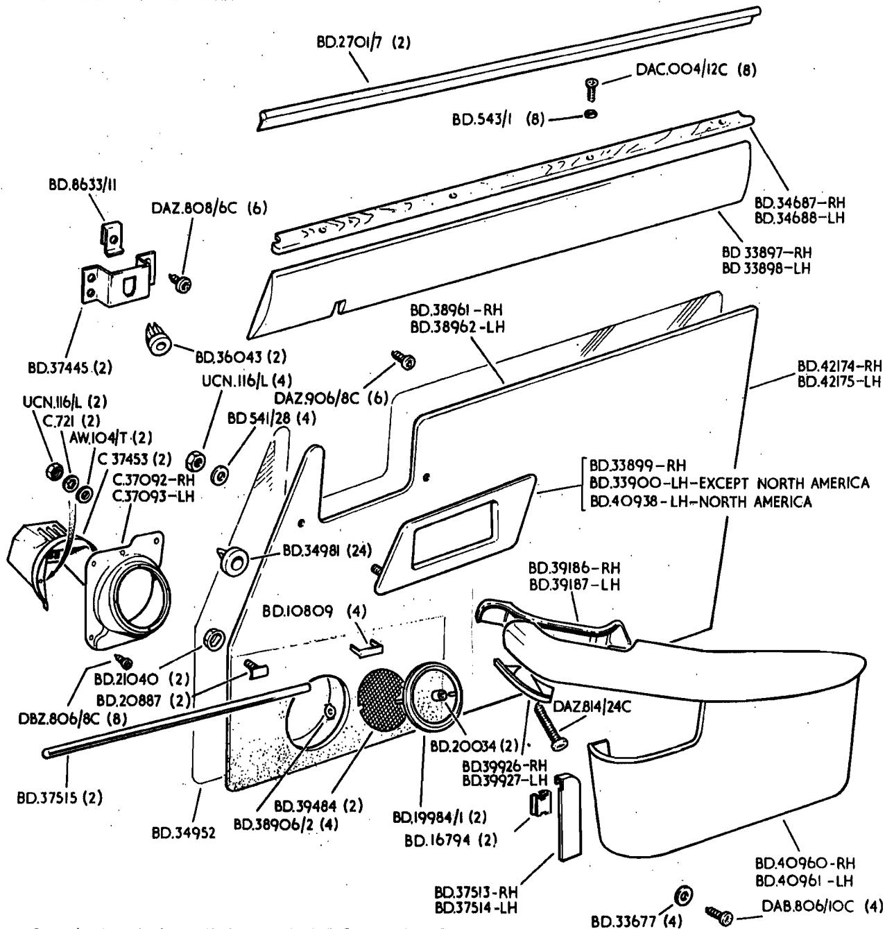
C.37506 ACOUSTIC DAMPING MATERIAL FOR C.37092 AND C.37093
